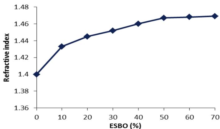
**Fig. 6. Effect of ESBO content on the refractive index of ESBO/DMU blends**
