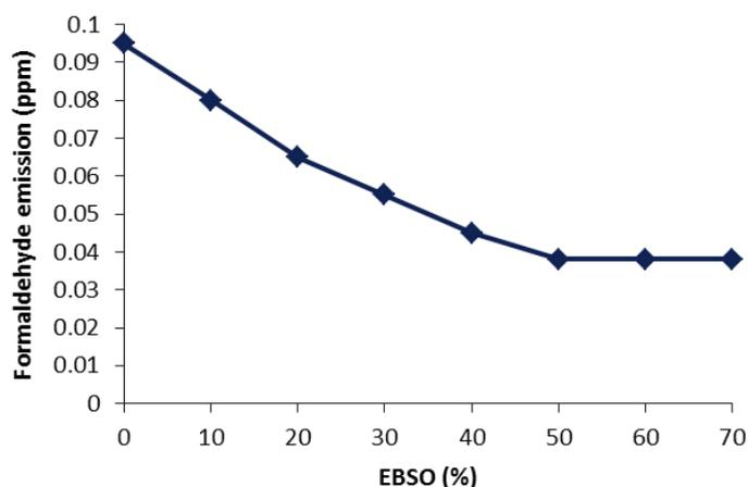
**Fig 10. Effect of ESBO content on formaldehyde emission of ESBO/DMU films.**
