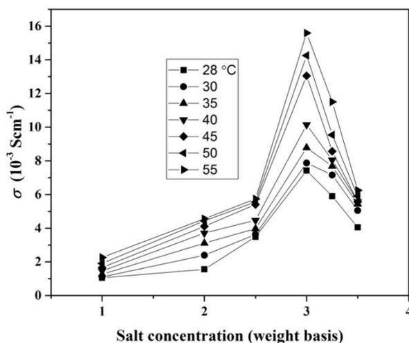
**Fig. 2. Conductivity isotherm curves for IL based GPE with different salt concentrations**
