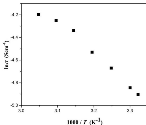
**Fig. 4. Variation of the natural logarithm of conductivity with 1000 / T for the optimized IL based GPE composition**
