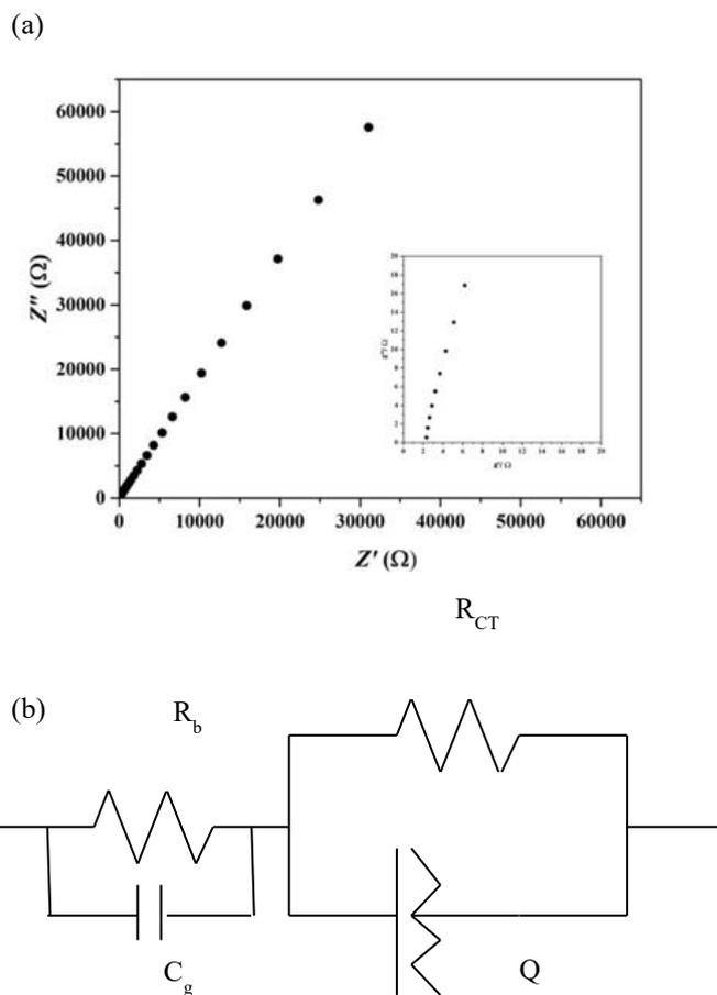
**Fig.1 (a) AC-impedance plot for PVdF-co-HFP:ZnTF:1E3MITF polymer electrolyte (Inset – expansion of high frequency region), and (b) Equivalent circuit of SS/IL based GPE/SS cell**
