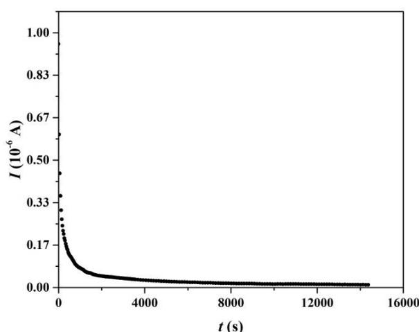
**Fig. 5. Current variation with time for the electrolyte with electrode configuration SS/ IL based GPE/ SS under 1 V DC potential**
