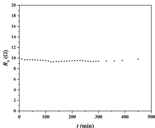
**Fig. 9. Variation of bulk electrolyte resistance ( $R_b$ ) with time**
