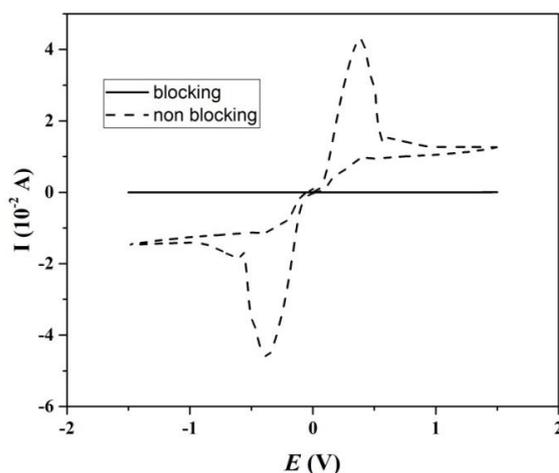
**Fig. 8** Cyclic voltammogram for cells Zn/ IL based GPE/ Zn and SS/ IL based GPE/ SS at a scan rate  $10 \text{ mV s}^{-1}$
