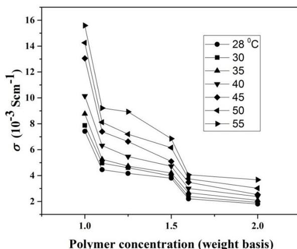
**Fig. 3. Conductivity isotherm curves for IL based GPE with different polymer concentrations**
