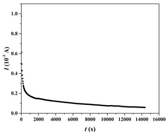
**Fig. 6. Current variation with time for the electrolyte with electrode configuration Zn/ IL based GPE/ Zn under 1 V DC potential**
