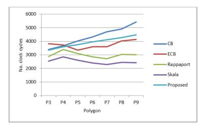
Fig 8. The number of clock cycles to clip against polygon windows
